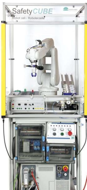
A photograph of a robotic workstation labeled "SafetyCUBE". The setup includes a white safety enclosure with yellow vertical supports. Inside, a white ABB IRB120 robotic arm is mounted on a silver base. The base unit contains various electronic components, including a control panel with buttons and a small screen, and a computer system. Cables are visible, connecting the robot to the internal electronics. The entire assembly is designed for safe operation in a controlled environment.
